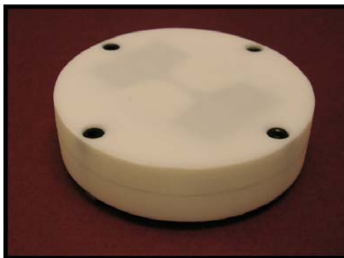
Figure 2: Custom-Enclosed “Hockey Puck” RF tag.
